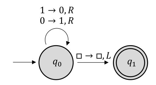
ID for the input string 0110  $q_0 0110$   $\vdash 1q_0 110$   $\vdash 10q_0 10$   $\vdash 100q_0 0$   $\vdash 1001q_0 \Box$  $\vdash 100q_1 1$
