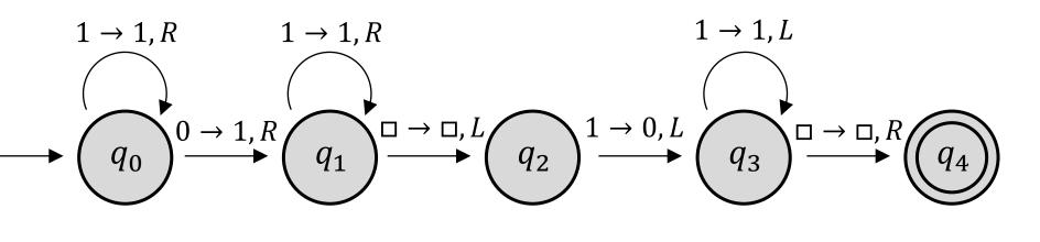
ID for the input string 3 + 2*q*<sub>0</sub>111011  $\vdash 1q_0 11011$  $\vdash 11q_0 1011$  $\vdash 111q_0011$  $\vdash 1111q_111$  $\vdash 11111q_11$  $\vdash 111111q_1\Box$  $\vdash 11111q_21$  $\vdash 1111q_310$  $\vdash^* q_3 \Box 111110$ ⊢ *q*<sub>4</sub>111110
