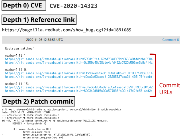
FIGURE 3: Example of where patches can be collected through the website provided by the CVE info page.
